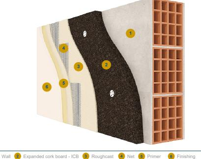
Overhead noise insulation (wall 22cm + 5 cm cork) = 50 dB Excellent thermal delay
